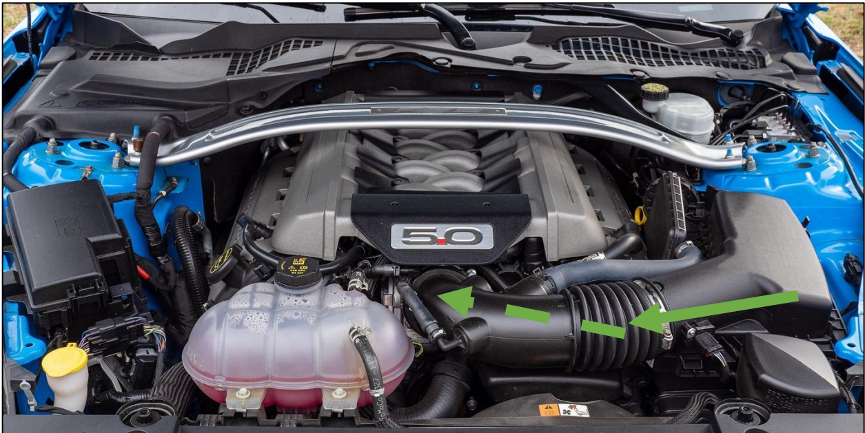
Image 23. Example 1 of Connection Point on Gas Engine
