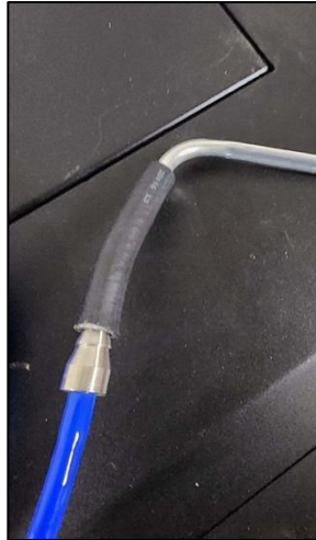
Image 28. Graduated Fitting Attached to Hose Adaptor
